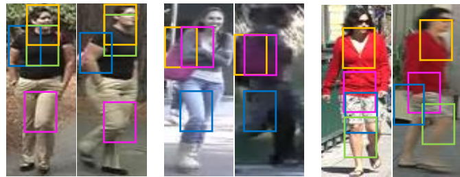
Fig. 9: Some visualized patch-wise graph matching results. In each pair of images, the bounding boxes with the same color refer to an established correspondence by our algorithm.
